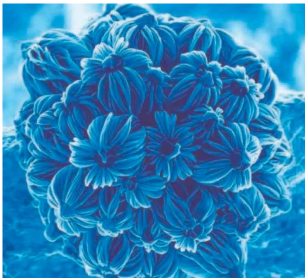
Figure 1. Blue nano-flower. Note: 3-dimensional Si composite nanostructures, taken with a scanning electron microscope, by Ghim Wei Ho. Image colour modified using the colour balance function in Adobe Photoshop. Source: Courtesy of and © Ghim Wei Ho and Professor Mark Welland.
