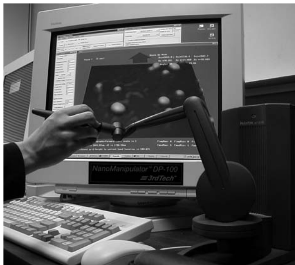
Fig. 3. 3rdTech's NanoManipulator adds 3D perspective and tactile feel to an atomic surface. (© J.N. England)
